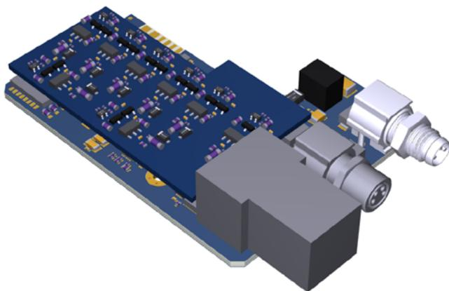
Figure 1: Prototype of a double circuit board; circuit boards placed on top of each other, CAD export
