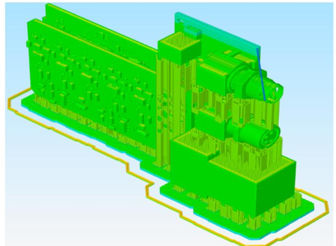
Figure 4: Slicer output for a circuit board. Overhangs must be supported by temporary supporting structures. They are broken off after the model is printed. The corresponding code, the G code file generated by the slicer, consists of ca. 400,000 lines of code.
